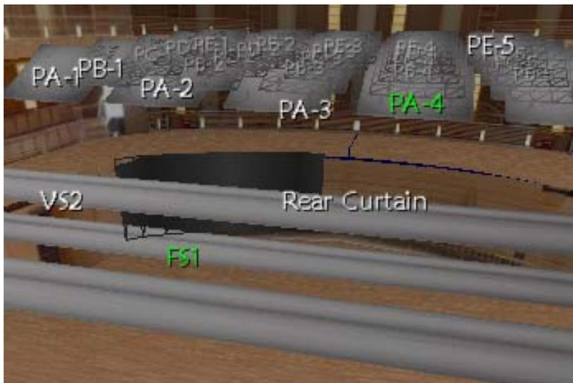
To select a set (or sets) for deadman operation, the operator touches the set label on the touchscreen. As an alternative, the operator can use the touchpad on the console to move the cursor and select sets for operation. Each set label will change from white to green to indicate that it has been selected.
