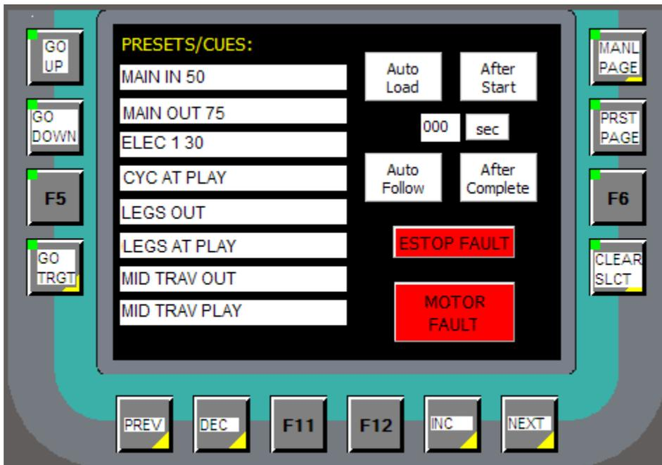
There are two indicators that will appear at the lower right of the screen if they are needed. ESTOP FAULT indicates that a system Emergency Stop button has been pushed. MOTOR FLT indicates that a system motor is in a fault condition. Use the main console screen to obtain details about which motor is in a fault condition.
