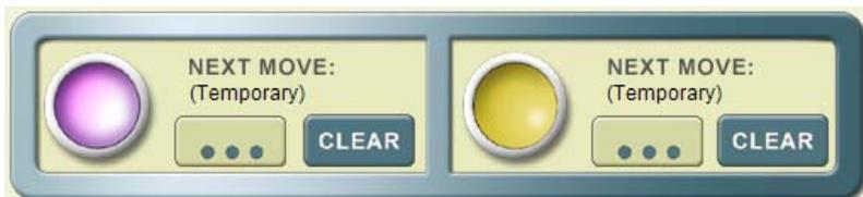
A preset is loaded onto one of the Go Preset buttons (violet or yellow). The operator can select a preset by touching the button with three dots next to one of the Go Preset buttons, and the list of
