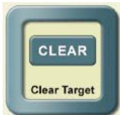
If a set has been selected and a target designated, you can undo the target designation by touching the "Clear Target" icon at the top of the screen. Clearing the target will clear the target wire-frame and the blue solid icon, and will return the set designation to a standard weight typeface
