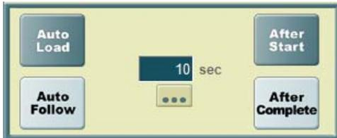
To execute an auto-follow move, the operator needs to continue holding the GO TARGET or DMB button through the move and the auto-follow timer. If the operator releases the button, the timer will stop, and the move will stop. Pressing the button again will continue the timers and/or the move from where it stopped.
