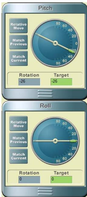
Some sets (e.g. acoustic panels) have three axes of motion – vertical position (raise and lower), pitch (tilt upstage-downstage), and roll (tilt stage left – stage right). When an acoustic panel is selected, indicators for vertical position, pitch and roll will appear at the right of the screen.
