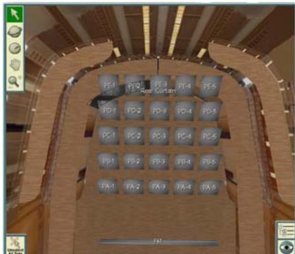
Touching the “Top View” selection on the list shown will shift the view to a plan view of the stage, as if the operator were on the grid looking down at the stage.
