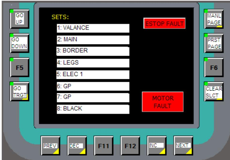
There are two indicators that will appear at the upper right of the screen if they are needed. ESTOP FAULT indicates that a system Emergency Stop button has been pushed. MOTOR FLT indicates that a system motor is in a fault condition. Use the main console screen to obtain details about which motor is in a fault condition.
