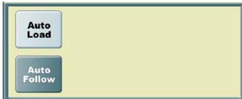
The top left button in the sequence box is Auto Load. This function is selected by default. If it is selected, and the current cue is run to completion, when the Go Target button is released at the end of the cue, the next cue will automatically load on the active Go Target button.
