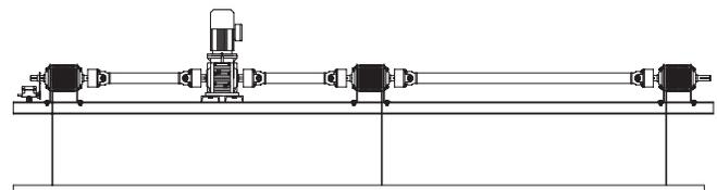
Figure 2. Line shaft winches are self-contained units with a separate drum for each lift line.
