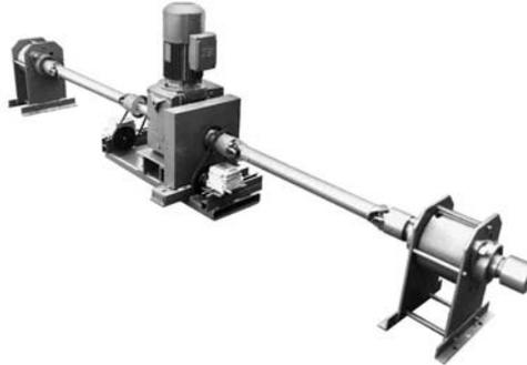
In order to prevent the batten from “walking” side to side as the lift line wraps on and off the drums, alternating right and left hand threaded drums are used.
